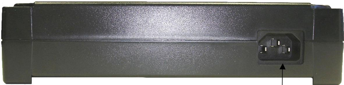
**Figure 3: Multiport Midspan AC Input**
