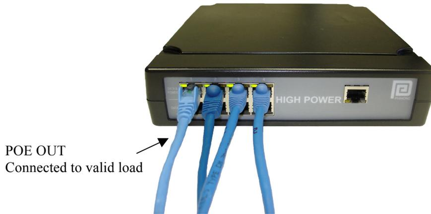
**Figure 7: Multiport Midspan PoE Connections**
