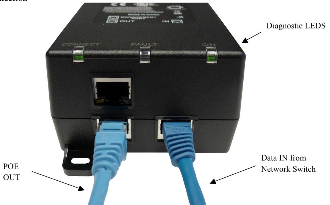
Figure 5: Single Port Midspan Data and PoE Connections
