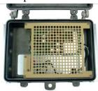
3) Connect cable glands (PGLAND750) or <sup>3</sup>/<sub>4</sub> NPT conduit piping to the face of the midspan. Ensure that connectors are fully installed to guarantee waterproof operation.
